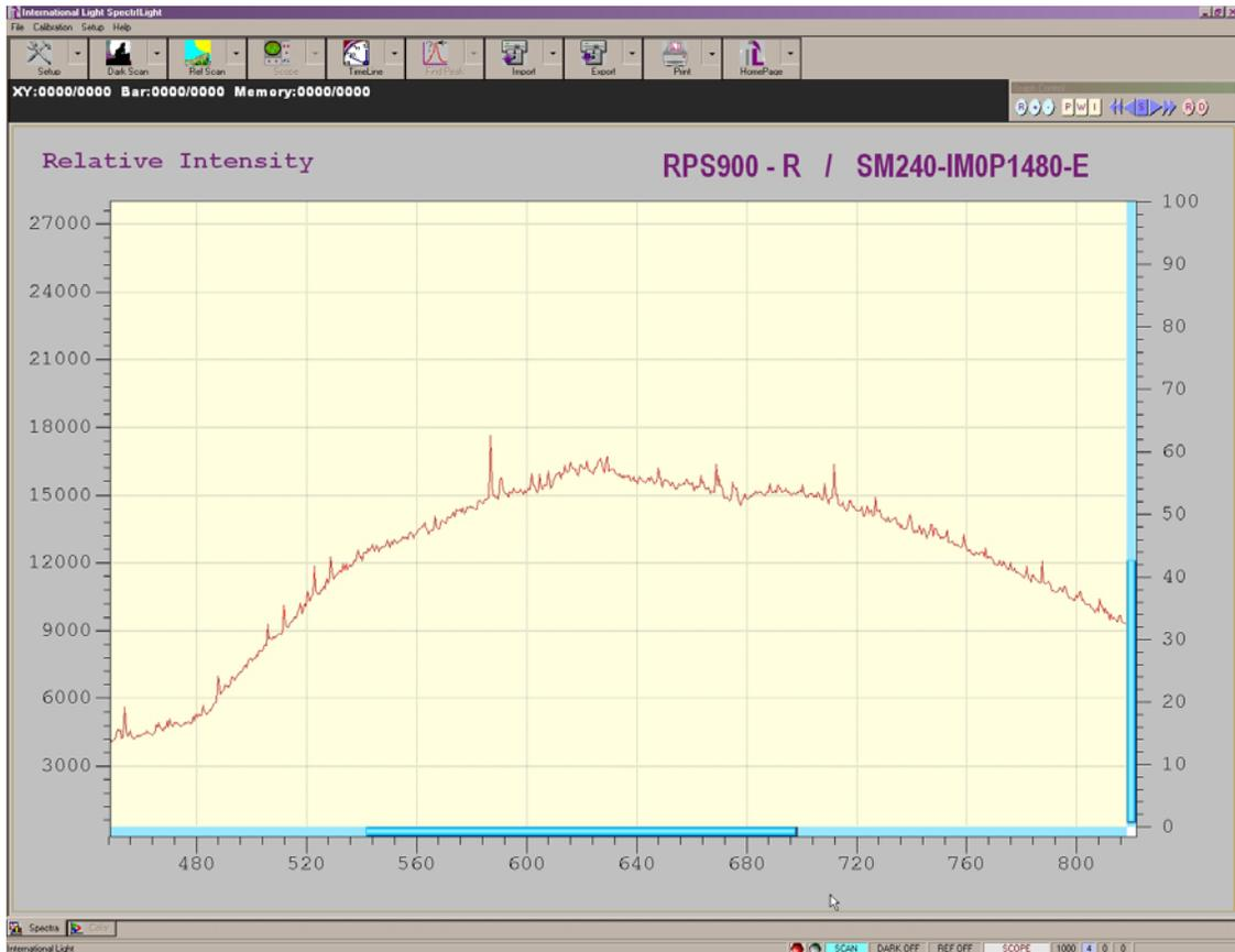
After a graph is zoomed in, two sliding bars will appear for vertical and horizontal scroll control use. Move the mouse pointer to any of the sliding bars until the pointer changes to a double arrow. Click and hold down the left mouse button and slide to view desired spectral display area in the graph.
