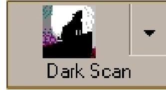
*In fact, the software does not permit selection of Irradiance mode unless a Dark Scan has been taken. To conduct a dark scan, first block all light from entering the spectroradiometer, and click the Dark Scan icon (not the arrow).*
