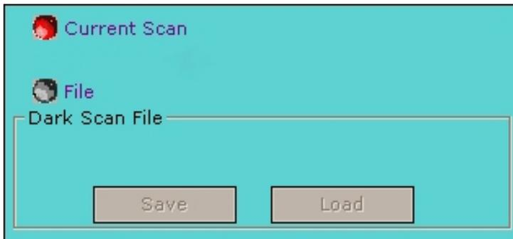
**Current Scan:** The current scan option is provided to take a dark scan from the current data that is being collected. This would be the normal setting for ILT900 Irradiance operation.
