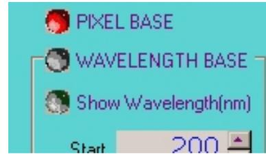
The peak is given to the nearest pixel. This mode is valuable in calibrating the instrument for wavelength, using discharge lamps or absorption standards.
