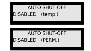
Press the 'INTEGRATE' button to 'INCREMENT' the bottom line between three choices: 'ENABLED (10 min)' for auto shut-off, 'DISABLED (temp.)' to temporarily disable the auto shut-off for one measurement session, and
