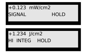
'HOLD': This message will blink in the 'status' register (lower right corner of the LCD) after the 'HOLD' button has been pressed, activating the 'HOLD' feature. The most recent reading will be frozen on the data display. To remove the 'HOLD' status, toggle the 'HOLD' button again or hit a function key ('SIGNAL', 'INTEGRATE', or 'ZERO') to select a new mode of operation.
