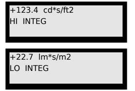
'HI INTEG' or 'LO INTEG': One of these messages is displayed continuously in the 'mode of operation' register (lower left corner of the LCD) after the 'INTEGRATE' button has been pressed, indicating that the instrument is in light integration mode. Press the 'INTEGRATE' button twice within one second to alternate between the 'HI' and 'LO' integration ranges. Press the integrate button once to reset the integral register in that mode to zero.
