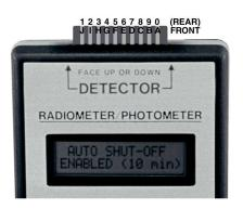
Request to Send ("RQSNDNOT") and Chip Select ("CSDM") are held low. An external button can be wired between "RQSNDNOT" and "GND" to provide remote sampling. When the switch is closed, connecting PIN 2 to PIN 4, the ILT1400 will send a continuous stream of data at a rate of one line (one reading) per second. The output is expressed in digital exponential notation. The ILT1400 transmits data once every 0.5 seconds.
