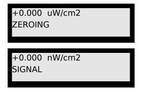
'ZEROING': This message is displayed temporarily in the 'mode of operation' register (lower left corner of the LCD) after the 'ZERO' button has been pressed, measuring the present light level and subsequently returning to 'SIGNAL' mode while subtracting this ambient light from future readings.
