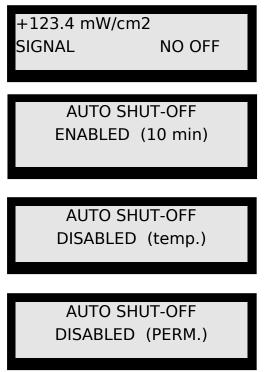
The first menu screen the user encounters in 'PROGRAM' mode is 'PROGRAM MODE', 'ON/OFF TO EXIT'. When the 'MENU' (ZERO) button is pressed, the display scrolls to one of the 'AUTO SHUT OFF' screens portrayed above. When the 'INCREMENT' (INTEGRATE) button is pressed, the bottom line of the display changes between three different forms: 'ENABLED (10 min)',
