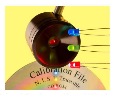
A new LED photometric detector that measures CIE averaged LED intensity per CIE 127-1997 Conditions A & B and provides calibration curves on a CD is being introduced by International Light.
