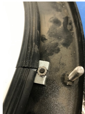
Fig 7. Line up rubber gasket seam with first lens clip.
