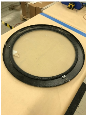
Fig 1. Remove entire flange and glass lens hanger.
