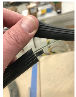
Fig 4. Remove rubber gasket from glass lens.
