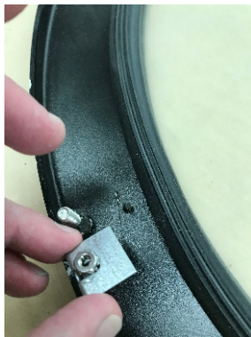
Fig 2. Remove lens clips.
