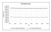
**W/A2 Diffused Quartz Head** with SMA adaptor for measuring spectral and total irradiance, illuminance, color parameters, and spectral characteristics of light sources.
