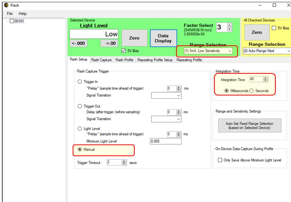
Figure 11. Windows Flash application manual flash capture.
