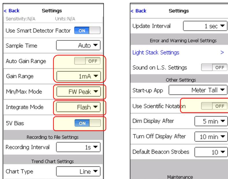
Figure 6. ILT2500 settings for flash measurement.
