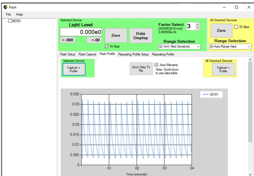
Figure 19. 500Hz flash capture, 1mA range.
