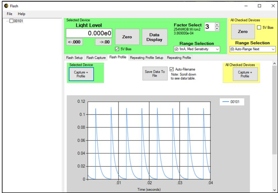
Figure 18. 200Hz flash capture, 1mA range.
