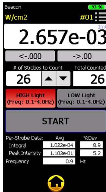
Figure 22. Flash capture with ILT2500 Beacon Applet.
