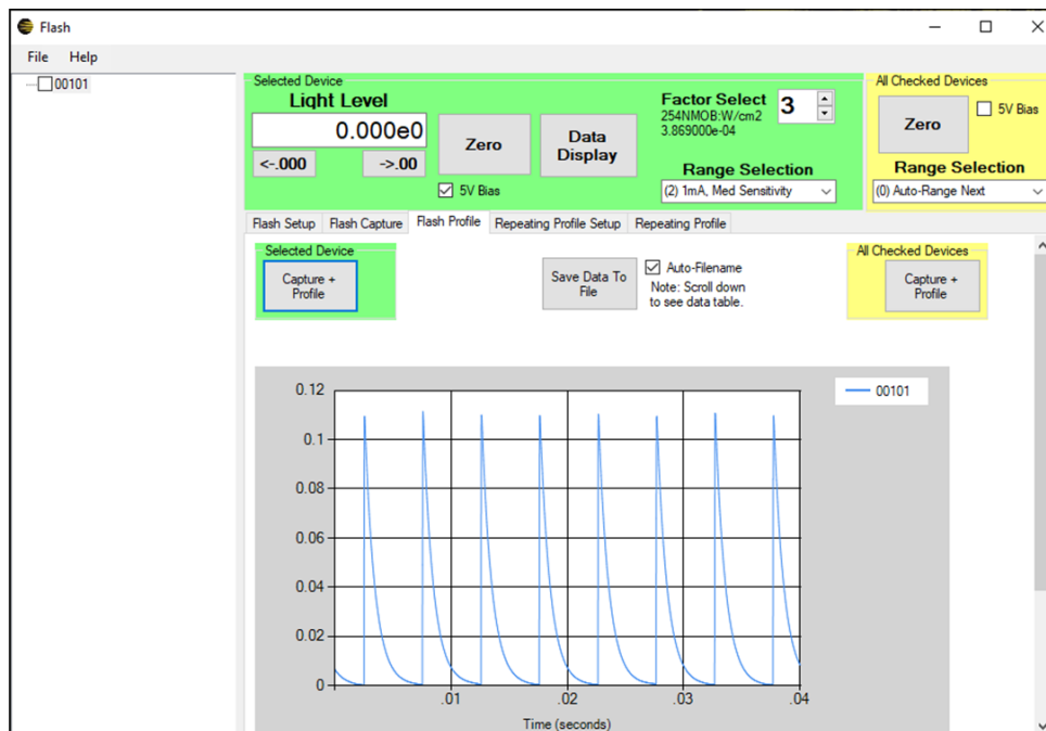
Figure 18. 200Hz flash capture, 1mA range.
