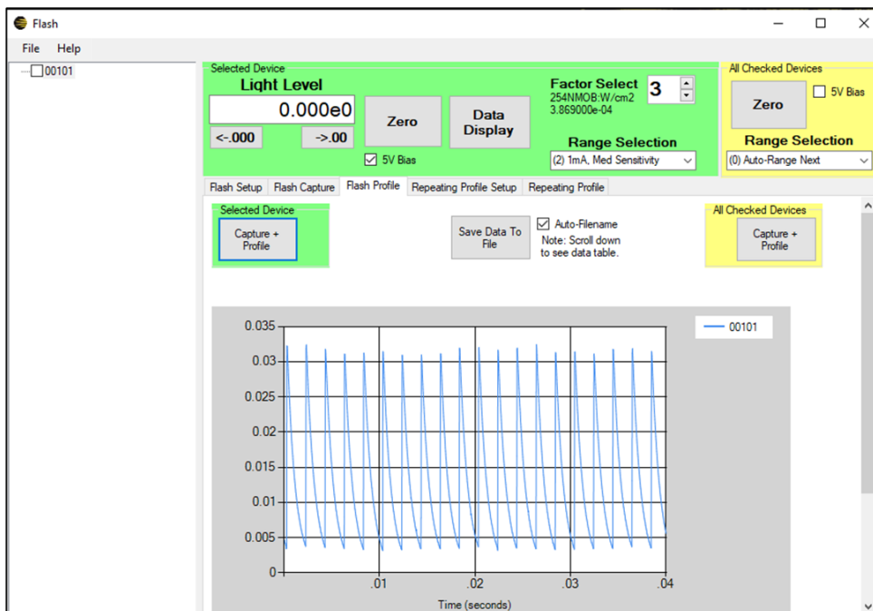
Figure 19. 500Hz flash capture, 1mA range.
