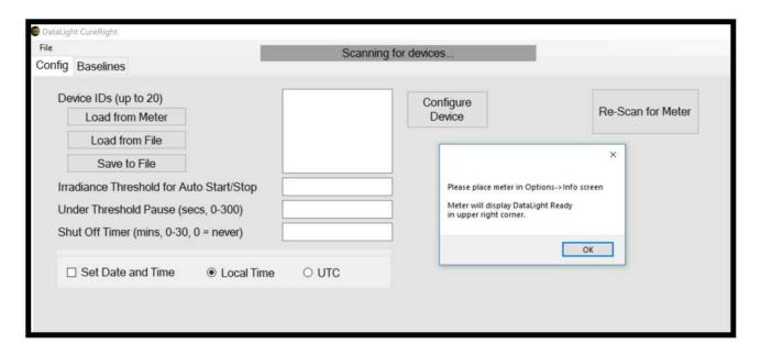
(note you can perform these steps in any order, If you initiate software first and when see a no devices connected error message, simply plug in the meter, turn it on, place in Data Ready Mode and then "Re-Scan for Meter" in the software.)
